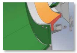
Spillage free mixer charging with no maintenance urethane seal
